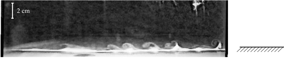
FIGURE 8. A video frame illustrating the vortex tubes in side view at \omega t = 105.7^\circ . U_{0m} = 43.9 \text{ cm s}^{-1} , T = 9.2 \text{ s} , Re = 2.8 \times 10^5 .
